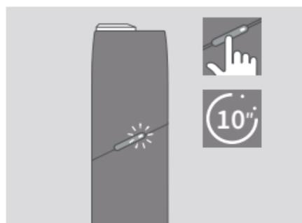
Press and hold IQOS Multi Button for 10 seconds then release; Battery Status Light and Button & Status Light will fade in, blink twice, then progressively fade in to confirm a reset.
